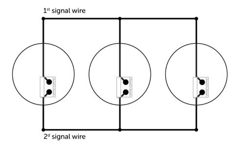
It is recommended to connect no more than 10 sensors in one line with a wire length of no more than 50 meters.
